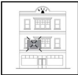
3. Sign conflicts with architectural features
